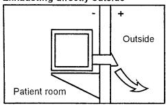
When ceiling mounting isn't an option, ducting directly outside or through a wall or window, the EX will satisfy that requirement.
