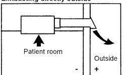
The ExC is designed for placement in a drop ceiling Exhausting into a duct system is permitted as long grid. Room exhaust can be directed outside, and is as the air is HEPA filtered first. This approach will permitted by CDC guidelines as long as air is filtered using a HEPA filter.
