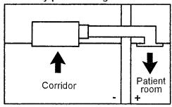
To create positive pressure, an ExC can be positioned outside the room and ducted into the room providing HEPA filtered air.
