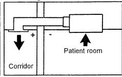
Exhausting back into the corridor will further positively pressurize the corridor while allowing the room to remain negative. Check with local building local fire codes.
