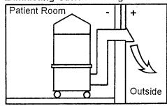
An oval duct for flexible hose or duct attachment for window exhaust.
