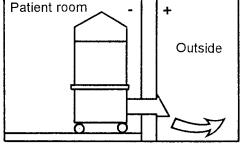
Through-the-wall rectangular exhaust duct.
