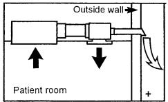
exhaust air can be sent outside, while the balance be done with a rectangular or oval duct attachment, air from outside the room and exhausting HEPA can be returned into the room. A damper control adjusts the flow through either duct.
